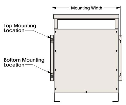
To mount the unit on the wall, first install two bolts (not included) on the desired wall at the correct mounting width apart and at your desired height (Minimum bolt size is 5/16" and of a suitable length and type for the intended mounting surface). Hang the transformer like a picture from these bolts at the top mounting locations. Next install two bolts with washers at the bottom mounting locations. Then (ONE AT A TIME) remove the top bolts to add a washer and re-install them.
