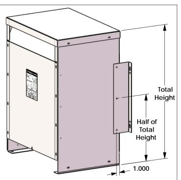
To attach wall mount brackets, put one of the included 5/16 x 1" self-drilling/tapping screws through the center hole of the wall mount bracket and through the case. It should be 1" from the rear of the case to the hole and at the centerline of the cases vertical height. Then add the other 2 adjacent screws. Repeat for other side.
